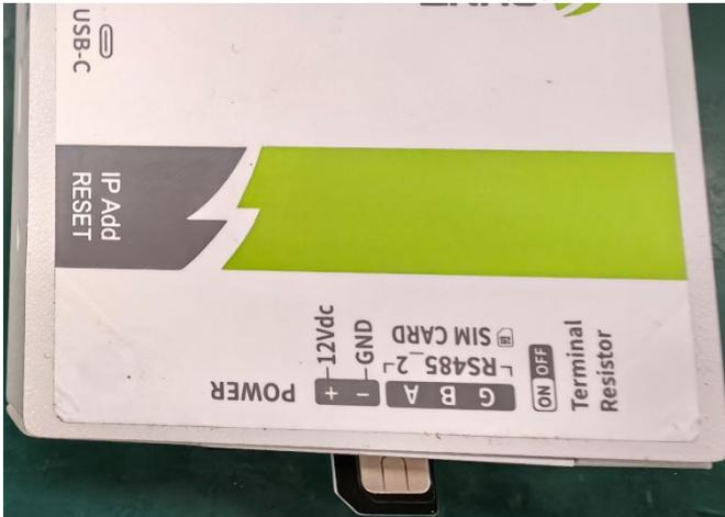
Figure 4- 21 Insert SIM card
