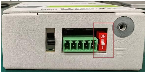
Figure 4- 22 Set DIP switch of MatriCloud Gateway
