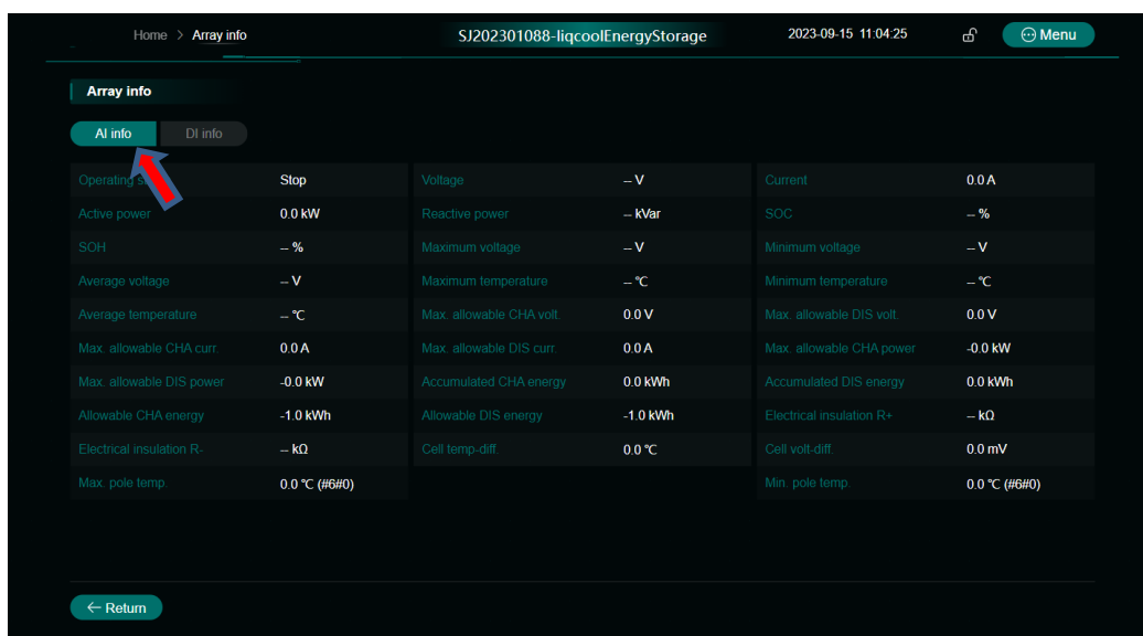
Figure 7- 3 Display of Multi-cluster Parameters on HMI (for reference)
